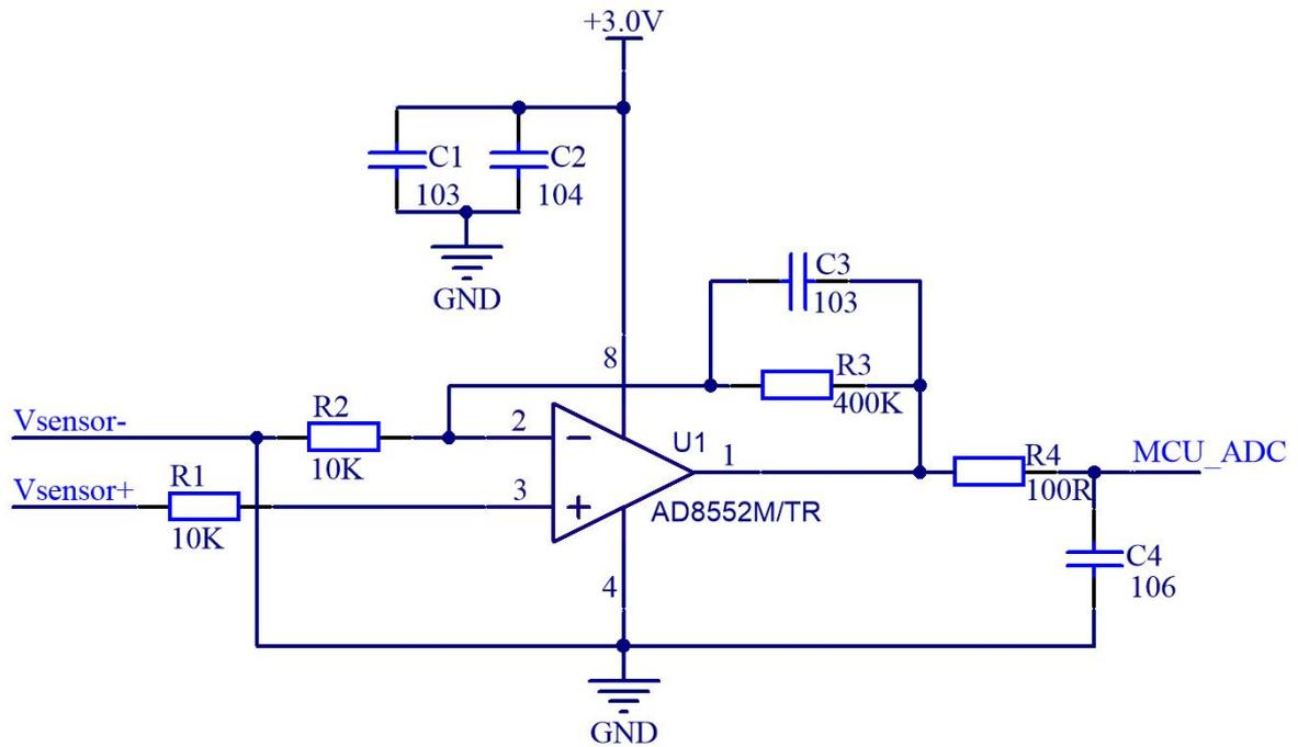
Figure 3. AO-06 recommended application circuit diagram
