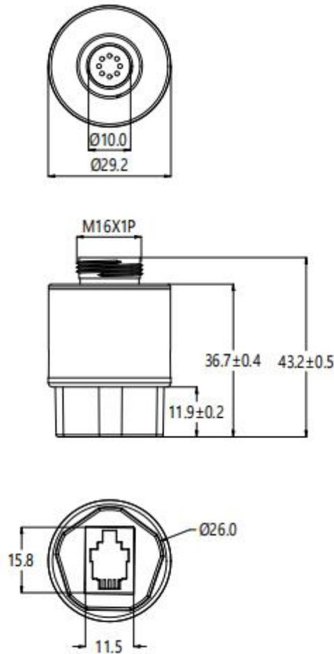
Figure 2. AO-06 outline dimensions (unit: mm, other unmarked tolerances:  $\pm 0.2$  mm)
