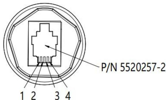
Figure 4. AO-06 pin definition diagram
