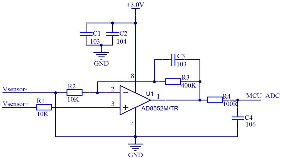
Figure 3. AO-09 recommended application circuit diagram
